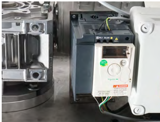
Electronic frequency converter in P models
